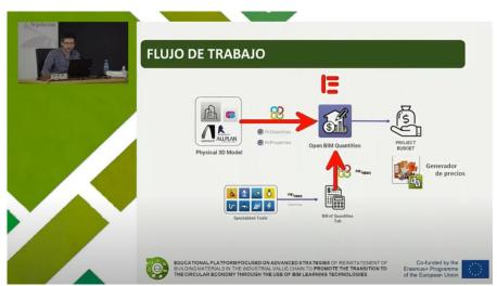
The project workflow, which uses the BIM model and the basis for constructive solutions, was explained. First in a theoretical way, and then in a practical way with an example of the CYPE Architecture tool and Open BIM Quantities, showing how to modify building elements step by step and generate the economic and energy costs and waste generated.
